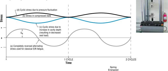
There are several types of loading that can result in fatigue failure, the most common type being alternating tension and compression or reversed loading. Loading of this type is illustrated in line (a) in the figure above, and is the type used in fatigue testing to develop the endurance or fatigue limits ( $S_e$ ) of materials. The endurance limit is the stress below which fatigue failure will not occur, regardless of the number of applied cycles (generally considered 10<sup>7</sup> cycles).
